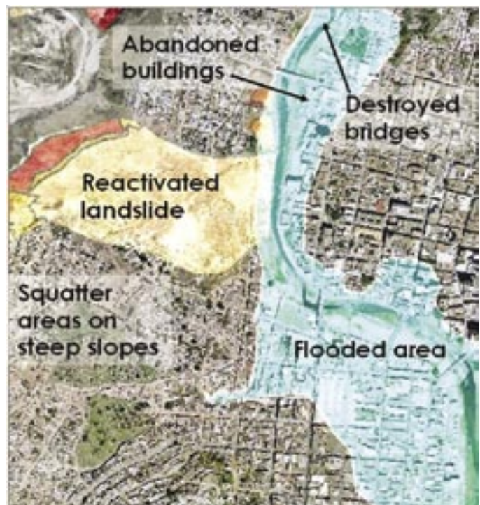
Figure 1. High-resolution image of the center of Risk-City with some of the hazard and vulnerability features indicated
